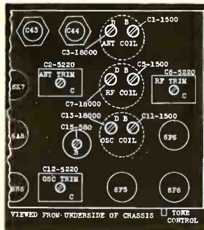
Underside view of G-E A-83 and A-85 sets giving alignment frequencies and location of padding condensers.
